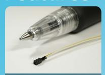
Fujikura's miniature CMOS image sensor modules combine miniature color CMOS image sensor with wafer level optics and micro coaxial cables.
